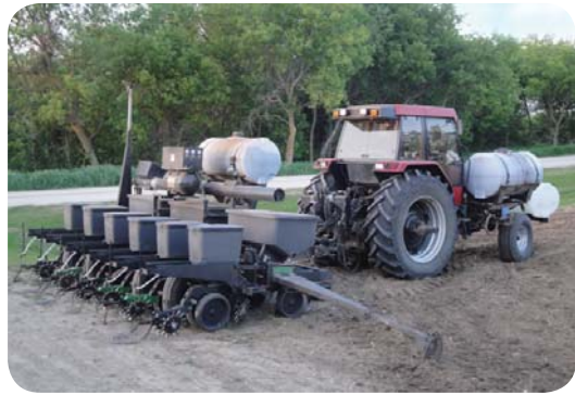
New Concept Planter for the U-Trough Approach Placement of Nutrients
